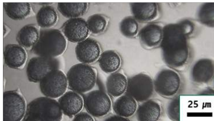
Fig. 1. Optical microscope photograph of QD colloid microcapsule
